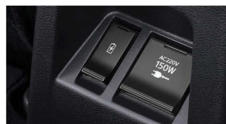
AC POWER OUTLET 220V/150W 2
